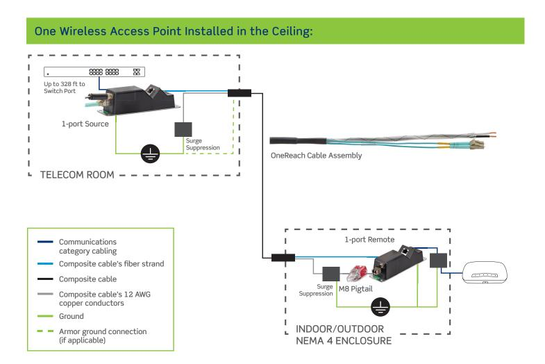
Combining optical fiber for long-distance data transmission and copper conductors in a single system takes PoE up to 10,000 ft.\* and PoE+ up to 5,000 ft.\*
