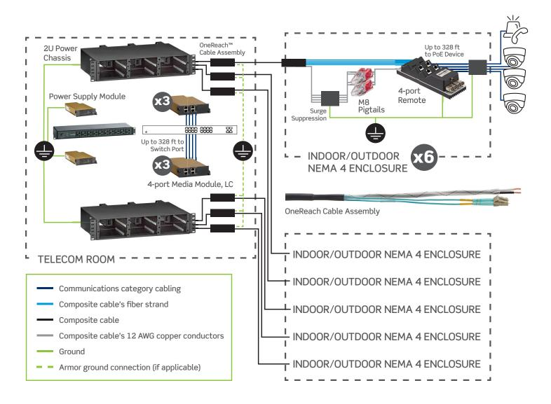
The following two tables provide the supported distance between the head end (1-port sources, media modules, and/or chassis) and the Remote PoE Ports, using 12 AWG composite cables to connect the ends. The first table is for use with the 1-port Remotes; the second table is for use with the 2-port and 4-port remotes.
